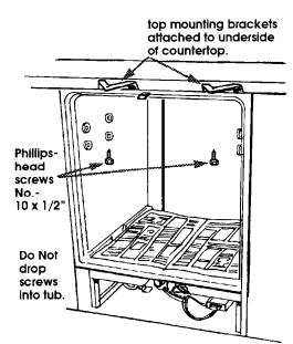
Open dishwasher door and remove all shipping materials. Remove bottom rack. Place a newspaper or large sheet of paper over bottom of dishwasher to protect the pump area when securing dishwasher to countertop.
